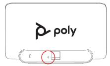
**3.** While continuing to hold the restore button, reconnect the LAN cable to power the device on. Don't power off the device until it finishes the factory restore process.
